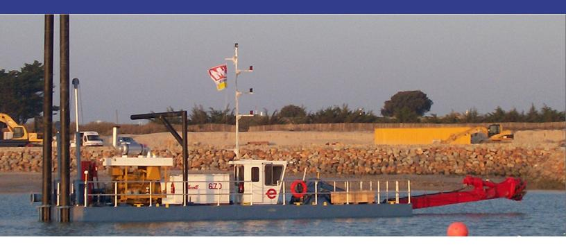
The 670 cutterhead dredge is a medium size, portable dredge.
